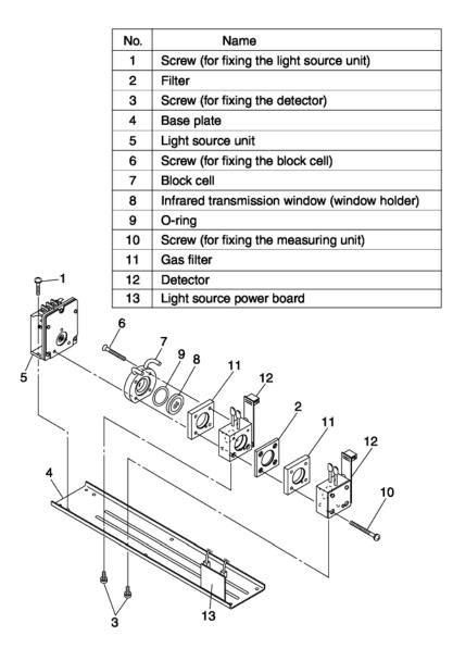
Figure 7-2: Measuring Unit Configuration (Block Cell)
